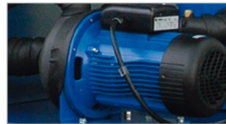
Single water pump with medium or high head pressure.
